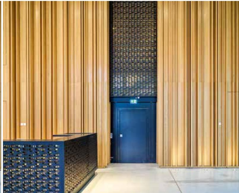
In daily operation, the fire sliding door is invisible. You would only see that it matches the colour of the perforated steel surfaces in the event of a fire.
