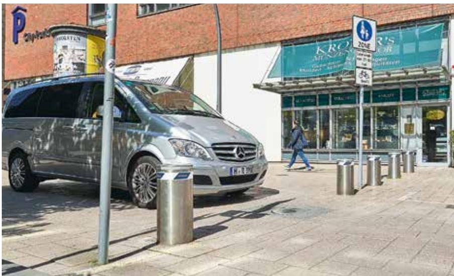
Authorised road users can let the bollard sink into the ground using a hand transmitter.
