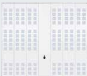
Style 988 Steel panel with ventilation slots (90 x 90 mm) Ventilation cross section: approx. 25 % of the door surface
